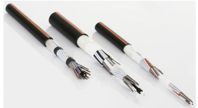
Datwyler's FO Outdoor cables are “virtually laterally watertight” due to the combination of HDPE sheath, swellable elements and gel-filled strands.
