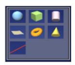
**PRIMITIVES**: sphere, cube, cylinder, cone and torus. These are used for object modelling. The plane is used as a construction tool (it has no substance!). The line thickness can be sized using the cursor size slider bar and for straight lines use the x, y and z keys.
