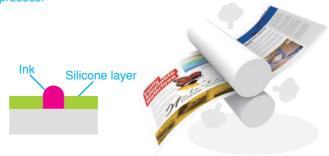
By eliminating the dampening solution from the printing process, the waterless printing system provides improvements in productivity, quality, and an environmentally-friendlier operation.
