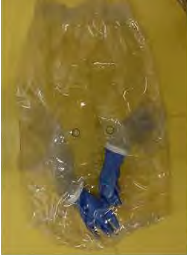
There are spray nozzles at the front and the back of the glove-change-bag to enable easy spraying of sleeve and clamps
