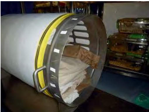
small pieces of tape are used to secure the foil tightly to the drum
