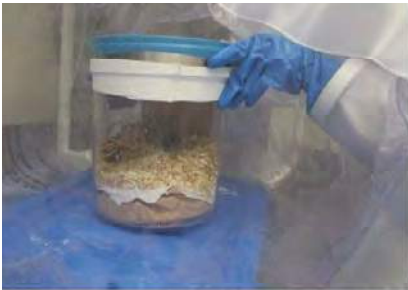
cages are placed inside the port bag and sprayed - one person holding and turning - second person spraying
