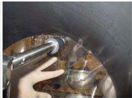
Special care is taken to spray the inner rim of the port cap. Push the cap inwards in order to reach right into the gap.
