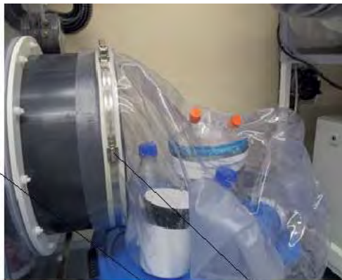
The bag is connected to the port and secured, using rubber band and clamp
