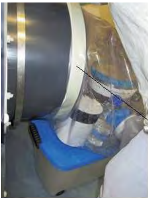
The bag is connected to the port and secured, using rubber band and clamp
