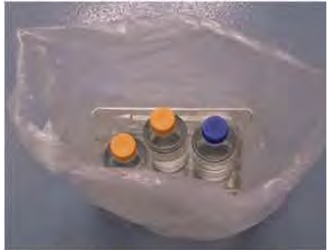
Bottles are placed into cage bottom or tray inside an autoclave bag.
