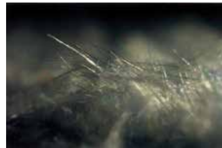
Microscopic, needle-like crystals fill the naturally occurring pores and capillary tracts of concrete for guaranteed waterproof structures.
