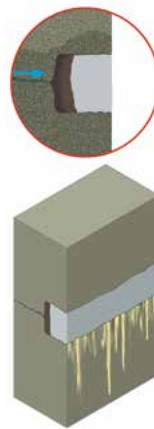
Step 3: Install Krystol Repair Grout.
