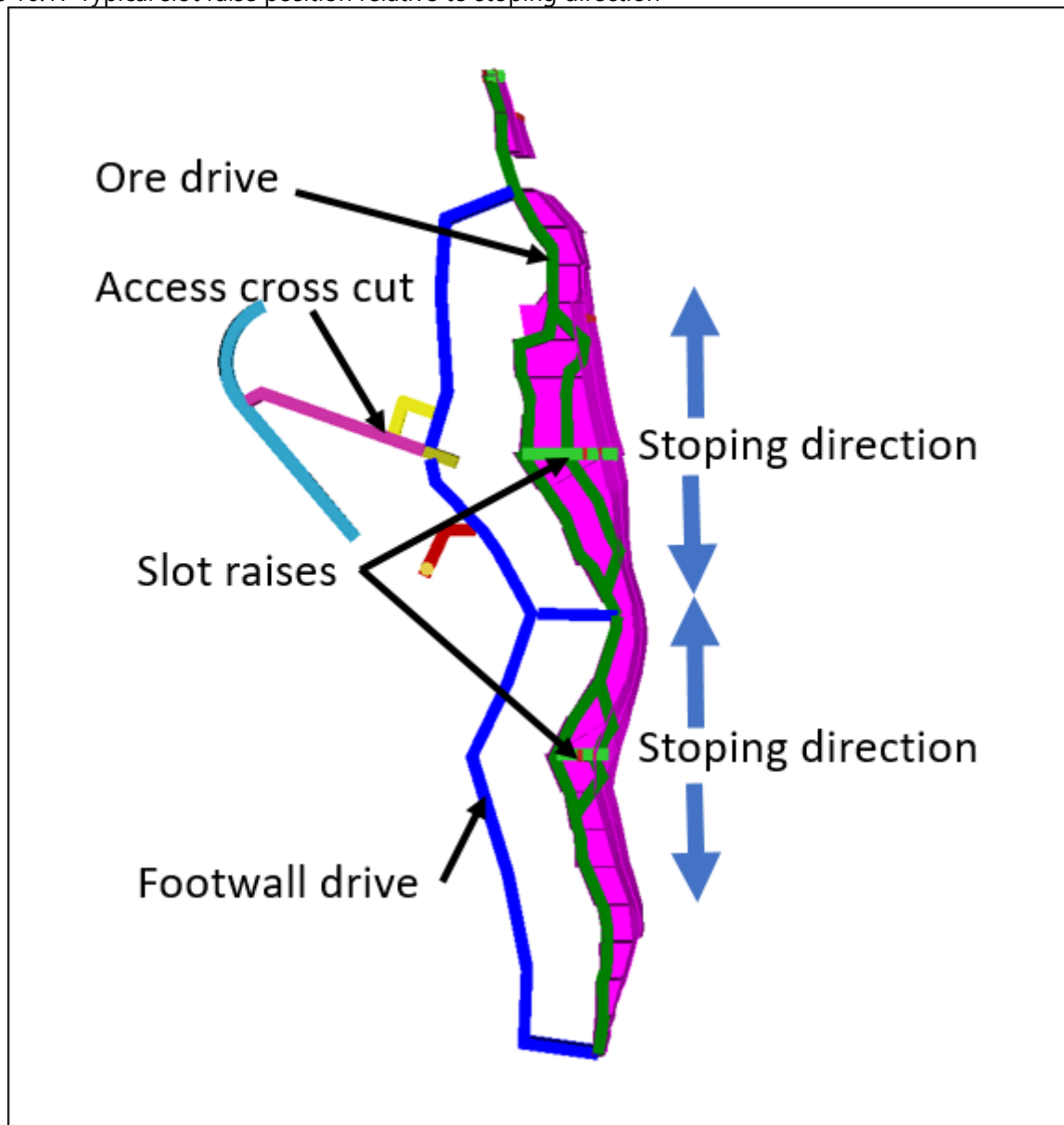
Figure 16.17 Typical slot raise position relative to stoping direction
