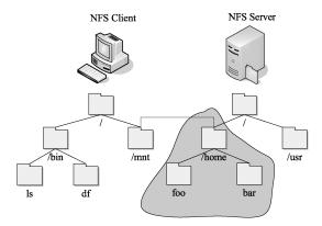
**Fig. 8.** NFS access control granularity with the (remote) mount protocol. The server exports a file system (e.g., /home) to the client. An administrator on the client mounts the exported file system (e.g., under /mnt). Because the server trusts the client to enforce file-access rights, object-access granularity in NFS is at the file system level.
