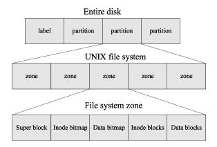
Fig. 4. On-disk layout of a typical UNIX file system (from [Farmer and Venema 2004]).
