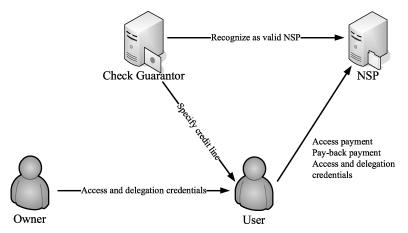
**Fig. 12.** A user wishing to access another user's file needs to have their own line of credit with a Check Guarantor (CG), as well as a credential from the file owner granting them access to that file. When accessing the file, the user needs to provide the credit-backing credential from the CG, a microcheck to the NSP, and the access credential(s) to the file. If the owner has set a "pay-back" disposition for the file, an additional microcheck to the owner may also be needed to gain access.
