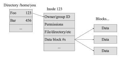
$\textbf{Fig. 3}. \quad \text{Simplified structure of the UNIX file system (from [Farmer and Venema~2004])}.$
