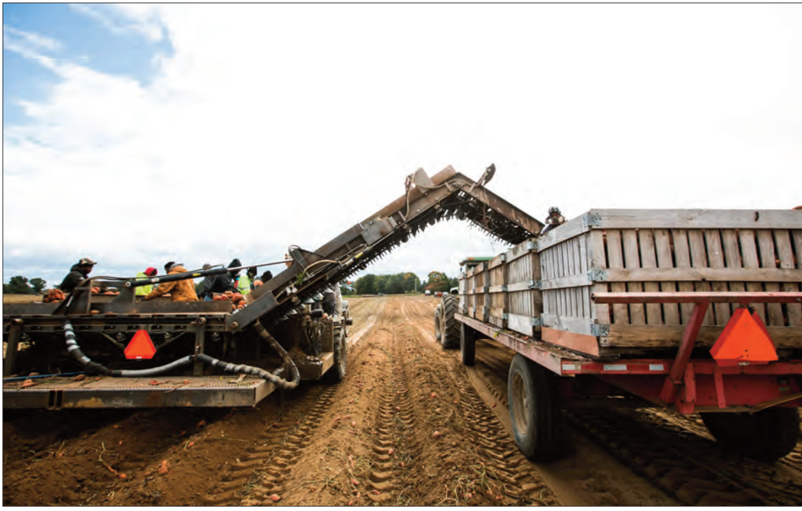
Sweet potatoes require capital-intensive, specialized equipment for planting and harvesting. Peter Jr. VanBerlo, Nick's brother, has expertise in fabricating what the farm needs to grow, pack and ship 25 million pounds per year from coast to coast.
