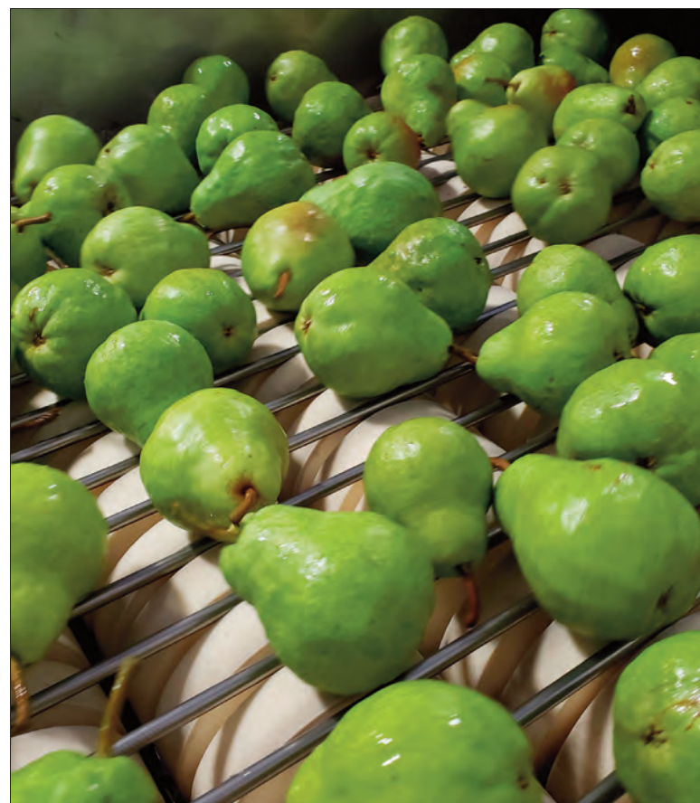
Pears are lifted several times with metal rods and set down to dry on rotating sponges to avoid scuffing the fruit. Photos by Myrna Stark Leader.
