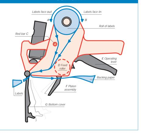
Feed end of roll with out facing labels in position (A).
