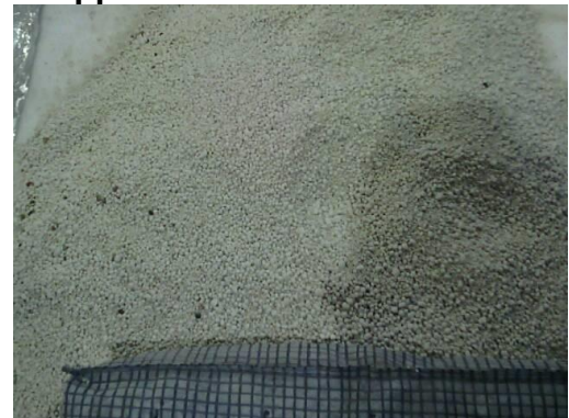
Visible Light Image – Released Beads covering the Cell Phone – suppressing fire, toxic gases and smoke.
