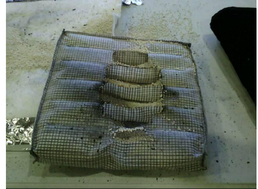
Visible Light Image – Beads were successfully released from the PED Pad
