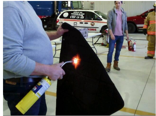
Visible Light Image – Torch flame applied directly to inner side (black) of blanket.
