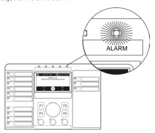
If the buzzer is sounding and the Fault LED is steady, then it's a fault.
