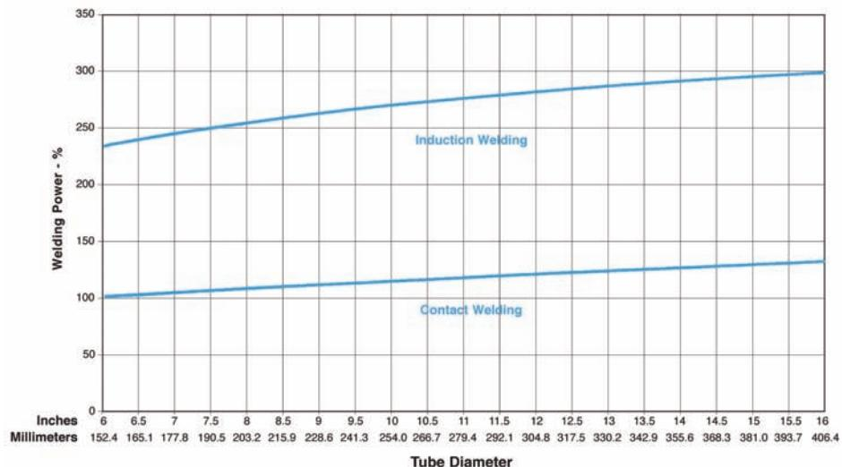
Note: Welding Power is for 0.5 Inch (12.5mm) Wall Pipe welded at 90 Feet per Minute (27mpm).
