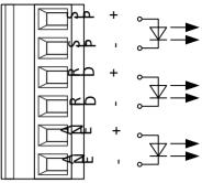
This terminal is used for control signal. This driver only accepts pulse/dir type signal (1-pulse input type).
