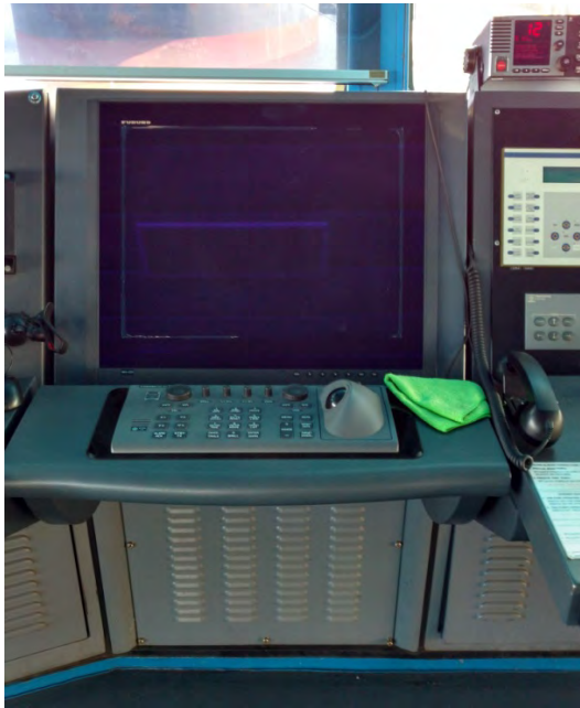
Fig. 5.3. a) The Furuno radar with ARPA on board the ship M/V Horyzont II b) the system for data registration
