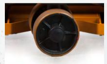
Polyurethane steer wheels and load rollers
