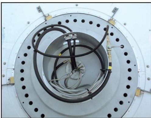
Robust brush holders that are designed to dissipate lightning energy and thus defend critical components
