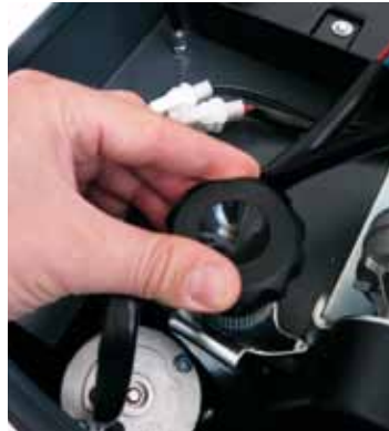
Main brush pressure adjustment
