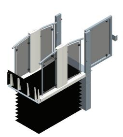
CLEARANCE EITHER SIDE OF STEPLIFT MUST BE <10mm OR >150mm TO COMPLY WITH BS6440.
