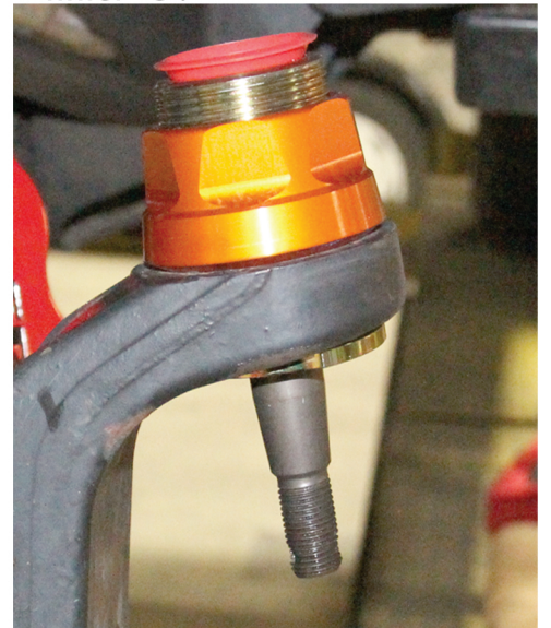
Install retaining nut using an adjustable wrench, or 2" socket . Torque to approx. 100 ft/lbs. TIP: Wrap the nut with painter's tape to protect the finish. If you need a 2" socket, we have one available (P/N: RP69248).
