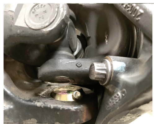
Install axle shaft and wheel hub. Ensure the axle shaft does not hit the lower ball joint grease fitting. To do this, rotate the axle shaft while turning the knuckle lock to lock.
