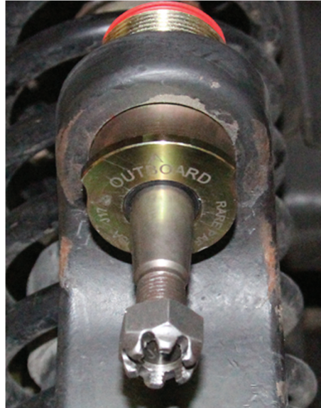
Ensure outer lip is facing outboard.
