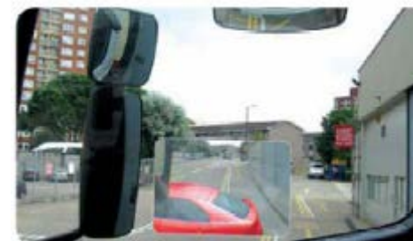
FRESNEL Lens showing a family saloon car in the lorry's blind spot.
