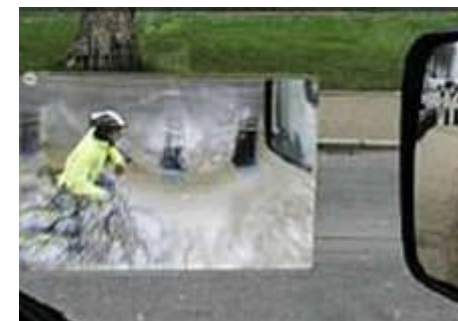
FRESNEL Lens showing a cyclist in the lorry's blind spot.
