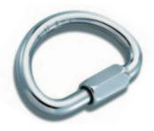
PPESCZ10 - Semi Circular Maillon Minimum Breaking Strain 45kN Maximum Gate Opening 10mm Certified to EN362
