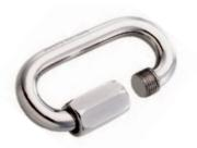
GOZ07 - Oval Maillon Minimum Breaking Strain 25kN Maximum Gate Opening 16mm Certified to EN362
