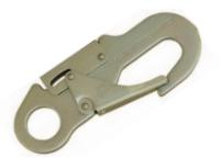
SH824 - Small Snap Hook Minimum Breaking Strain 27kN Maximum Gate Opening 21mm Certified to EN362
