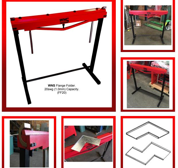
**WNS** 20swg (1.0mm) FLANGE FOLDER is the ideal machine when forming regular sized flanges. Designed to create a right angle flange on pre-cut sheet, this machine provides quick and easy folding of material up to 1.0mm thickness (mild steel). There is no need to keep measuring, nor clamping. The WNS Flange Folder also has the advantage of being 'open ended' allowing the user to also form inside flanges. Ideal for use with Pittsburgh Lock Rollformers.
