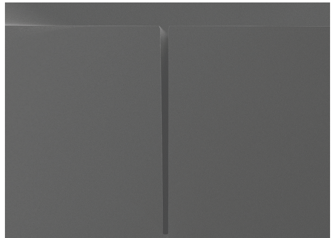
FIGURE 1. SEM image of TSI DRIE etch through silicon.
