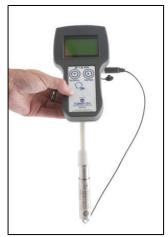
Jet Fuel Conductivity Meter (JF-1A-HH Model)
