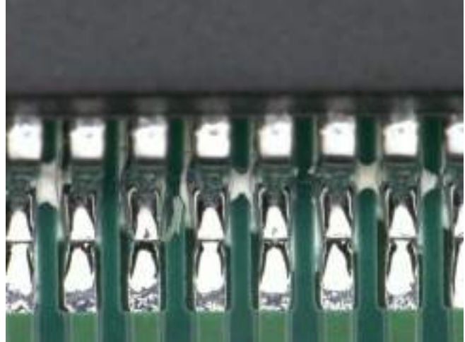
Figure 3: Visible White Residue after Cleaning
