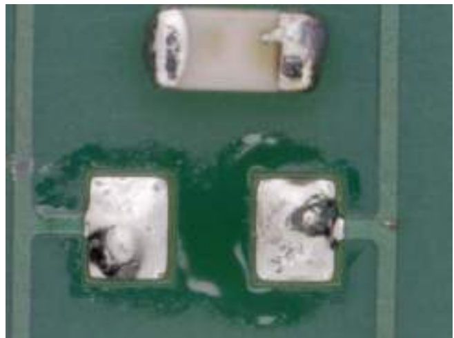
Figure 6: Flux Residue Bridging Conductors
