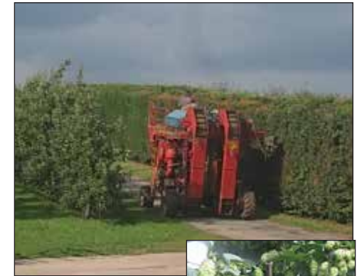
It's that man again! Duncan Reynolds driving a self-propelled machine for harvesting 'hedgerow hops', the shorter variety of hops grown on the farm.
