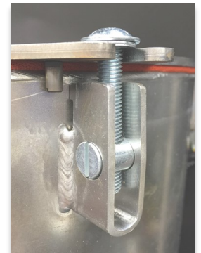
New 399 heat exchanger bolt design
