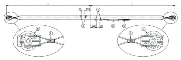
Assemble the Installation Pole (D) from the two parts using the split pin (A). Insert one pulley through the centre space (C) in the track, being sure that the back of the Pulley (B) faces the pocket. Using the Installation Pole (D) push the Pulley to the back of the pocket until it clicks into position. *Making sure that the cables are not twisted or crossing each other*, repeat for the second pulley, into the opposite pocket. Adjust the Cable-Tensioner (E) to the lightest setting.
