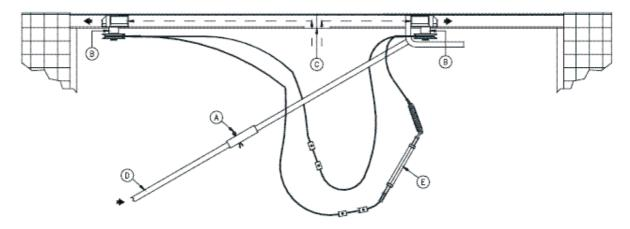
Fix the brackets (A) on the top of the doors – see (B) below. Hang the doors from the runners, and adjust accordingly. With the doors **centred** in the closed position, slot the cable into the brackets (A), fasten with screws (C), and tighten clips (D) (avoid over-tightening, as this will damage the cable). Adjust the Cable-Tensioner as necessary to fine tune the installation.
