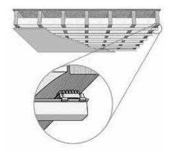
Remove original ceiling plasterboard (you also have the alternative if this is a lathe and plaster ceiling to leave the existing ceiling in place and screw through the ceiling to the joists. If you are considering this method then it is necessary to choose a 50mm acoustic mineral wool in the gap that you create. We suggest using the lighter flexible slab (http://www.soundstop.co.uk/ZEFSL50M.php)
