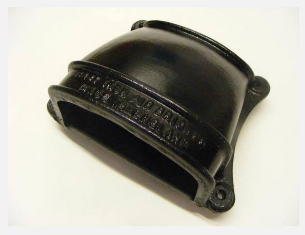
Cast iron conservation vents are made from grey iron, cast in sand moulds bonded with resin to a fine cast finish and are available in one size with two different diameter spigots at the back 100mm dia (4" item CON4) and 125mm dia (5" CON5) and also a the new heavy duty 150mm dia (6" CON6).
