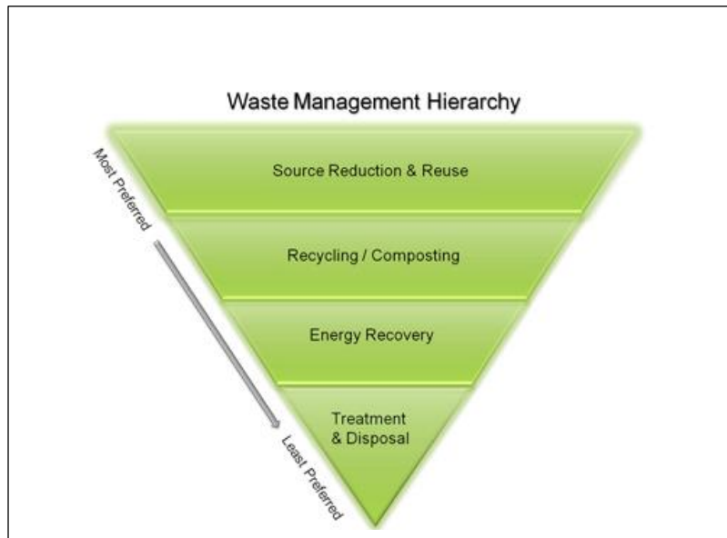
Figure 1. Zero waste hierarchy for the highest and best use of materials. Recycling / composting can include anaerobic digestion.
