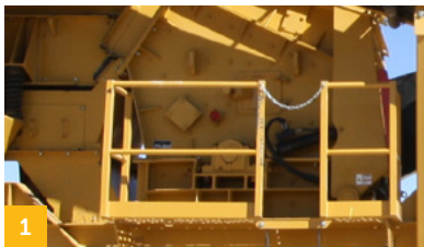
1 IROCK's four-bar rotor 4043 impactor design produces a consistent, uniform cubical product.
