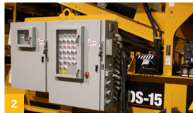
2 The RDS-15's on-board power source runs the complete operation as well as three auxiliary outlets.
