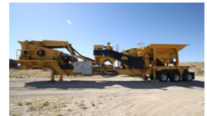
Closed-circuit design with a four-bar impactor offers exceptional durability and efficiency for producing uniformly sized product.
