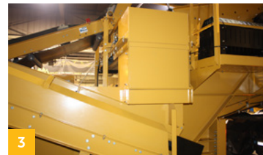
3 Ability to return top and middle deck oversized material back to the crusher. This feature increases production by splitting the load on two decks rather than one.
