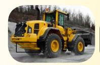
On wheel loader which work in quarry is neccesary to put on rear side aditional bottom counterweight to unload front tires.
