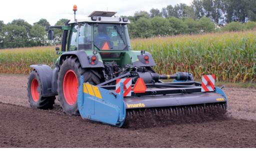
10% more capacity, 10% lighter in weight and 40% stronger through development are quite impressive. The re-design has also changed the appearance as the drive is now through a central gearbox from the pto to a secondary side gearbox driving the main digging rotor as opposed to the previous chain drive. This move inevitably reduces maintenance whilst increasing the strength and durability.
