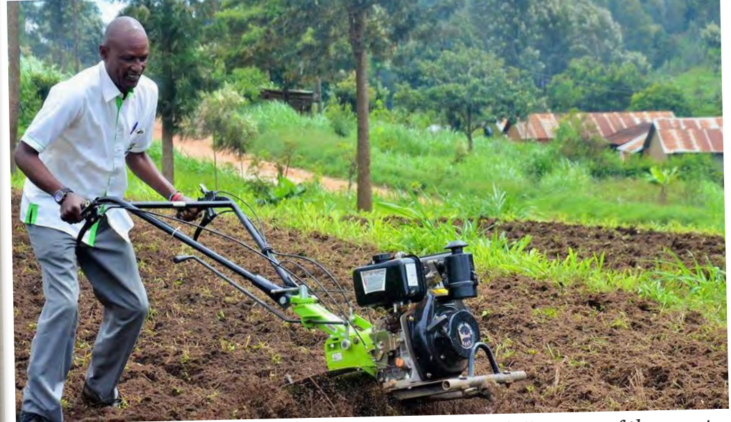
Multifunction power tillers for use by farmers in the hilly areas of the county
