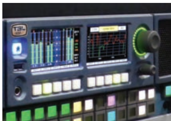
TSL Products' PAM1-IP and PAM2-IP audio monitoring units now include support for SMPTE 2110 and the Ember+ protocol.
