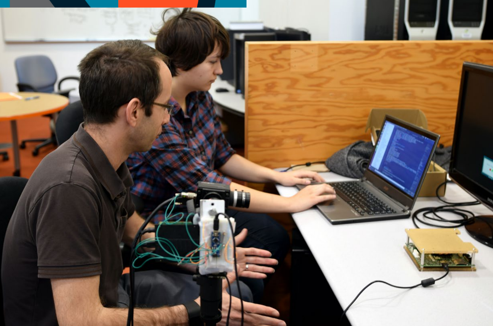
Course 6 senior Nicole Glabinski and postdoctoral researcher Guy Rosman work on her SuperUROP project, a “smart” 3-D scanner with the ability to change resolution and other parameters on-the-fly.
