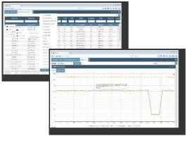
An SFP is an optical-to-electrical converter and ,as such, is subject to degradation over time. It is essential that these components are continuously monitored over time. The Transceiver View shows the current status along with the performance history of the SFP so you can see the device degradation over time and replace the SFP before performance becomes a problem.
