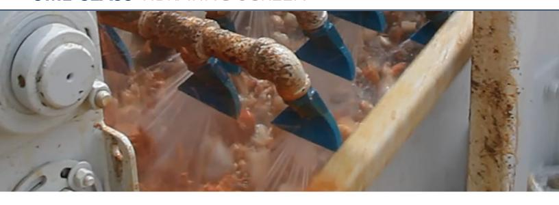
The Niagara UML-Class vibrating screen is a horizontal, linear motion screen built for light duty applications.
