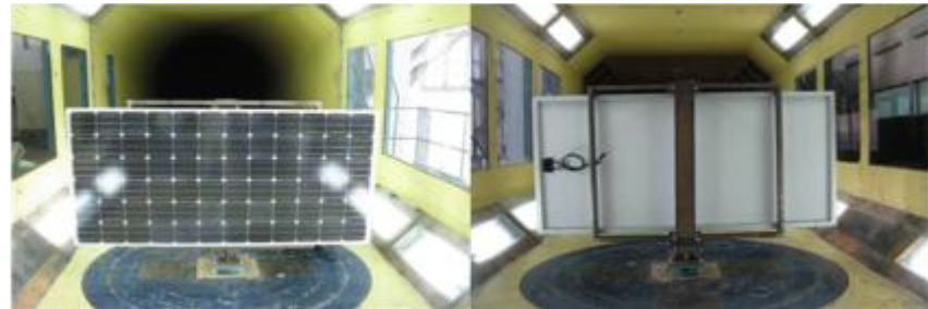
Modules installed by four clamps at long frame
