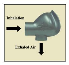
The check valves are replaceable if they become dirty or damaged. The valves are pressed into the respective ports and can be removed by applying pressure to the outer rim of the valve from inside the Nasal Mask. The inhalation and exhalation check valves are supplied by St. Croix Sensory as Part Numbers NR0041 and NR0042.
