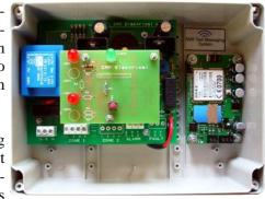
two inputs are energised. No phone lines are required just a SIM card from a mobile phone company that the users chooses.
