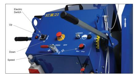
The desired cutting depth is adjusted by a motorized threaded spindle unit. In order to rise or lower the saw blade you use the electric switch on the left side of the machine panel. Turning the switch form his zero position in **two steps** to the left side and hold
