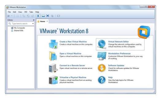
Click on Virtual Network Editor in the right pane of the VMware Workstation window. A list of virtual interfaces and the external connection to which they should be mapped is displayed.
