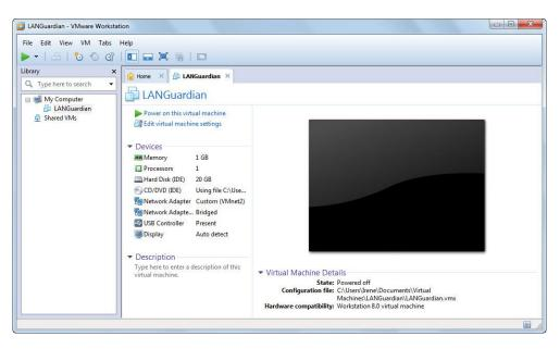
2. Select **Power on this virtual machine**. The installation of LANGuardian begins automatically and the LANGuardian Setup Utility is displayed.
