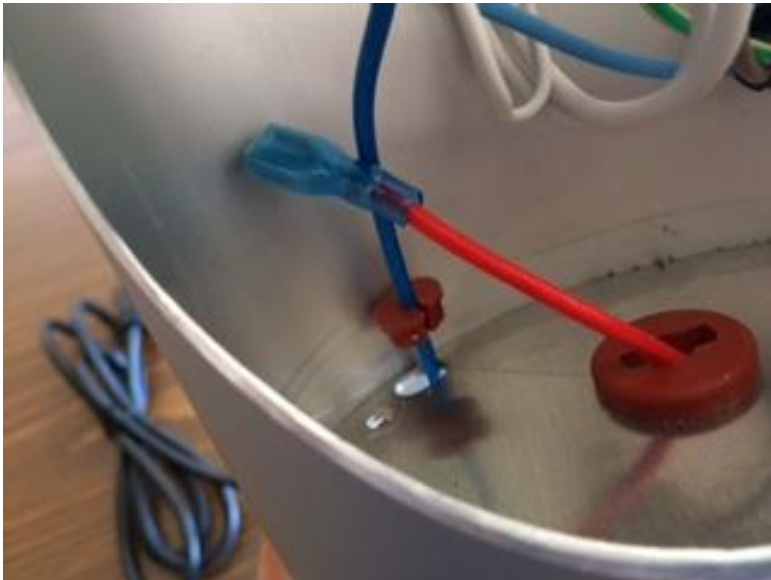
Step 5: Dismount silicone stopper on the cable
