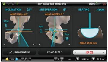
Fig 2. Real time cup impactor tracking with respect to the anterior pelvic plane and native acetabular rim. 3D position and seating depth relative to the last reamed position is also provided
