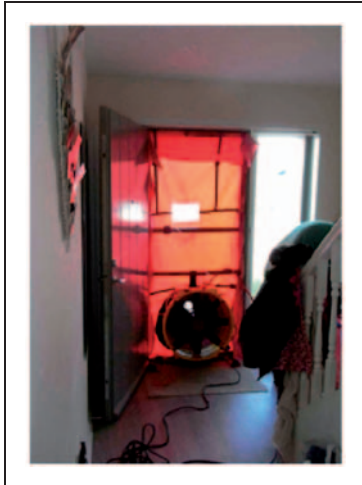
Figure 2. Tarpaulin fitted to the patio doors in the living room.
