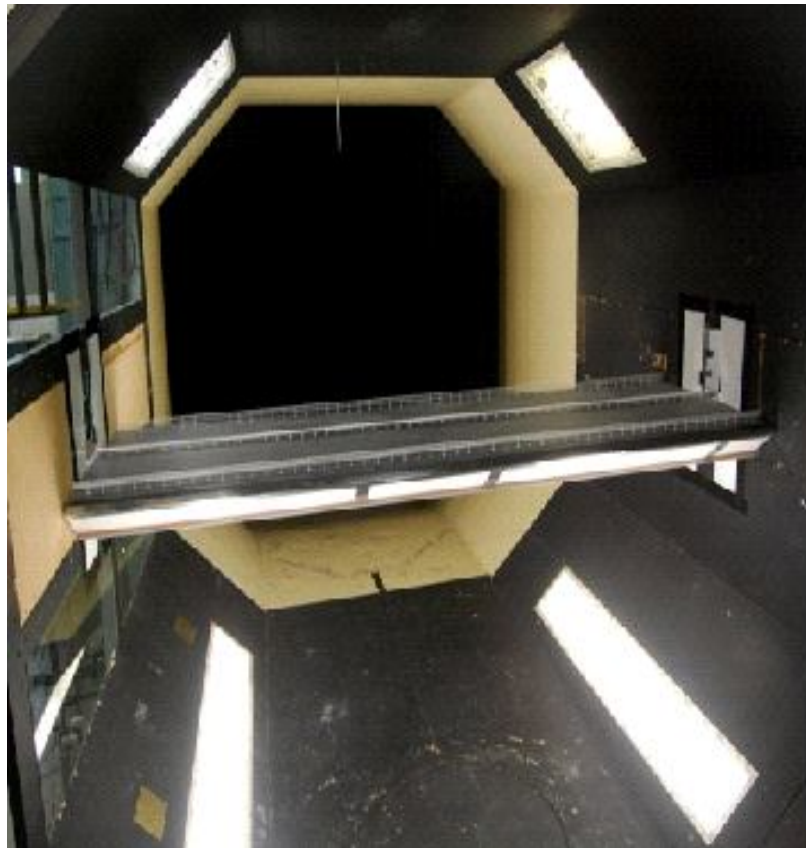
Wind Tunnel Model - General View
