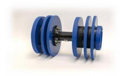
The scraping action of the sealing discs has proved successful in removing light deposits from the pipe wall; this cleaning ability can be further enhanced by the addition of brushes, plough blades or pin wheel discs. Other design options include the attachment of magnets (for debris collection), gauge plates and transmitter housings.
