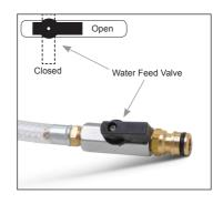
The water feed system is built into the machine. To connect with the water supply, first pull the quick-release collar to remove the female side of the water coupling. Then unscrew the nut and engage the coupling to the water hose. Now reconnect the water coupling to the male water feed valve. Press it until it clicks.
