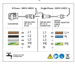
If more power is needed, and a 32A or larger breaker is available, the main plug may be removed, and the converter's main power supply cable may be directly wired to the breaker. In this case, connect the L1 and L2 wires to the breaker, leaving the L3 wire unconnected. Then connect the earth (ground) wire to the earth connection.
